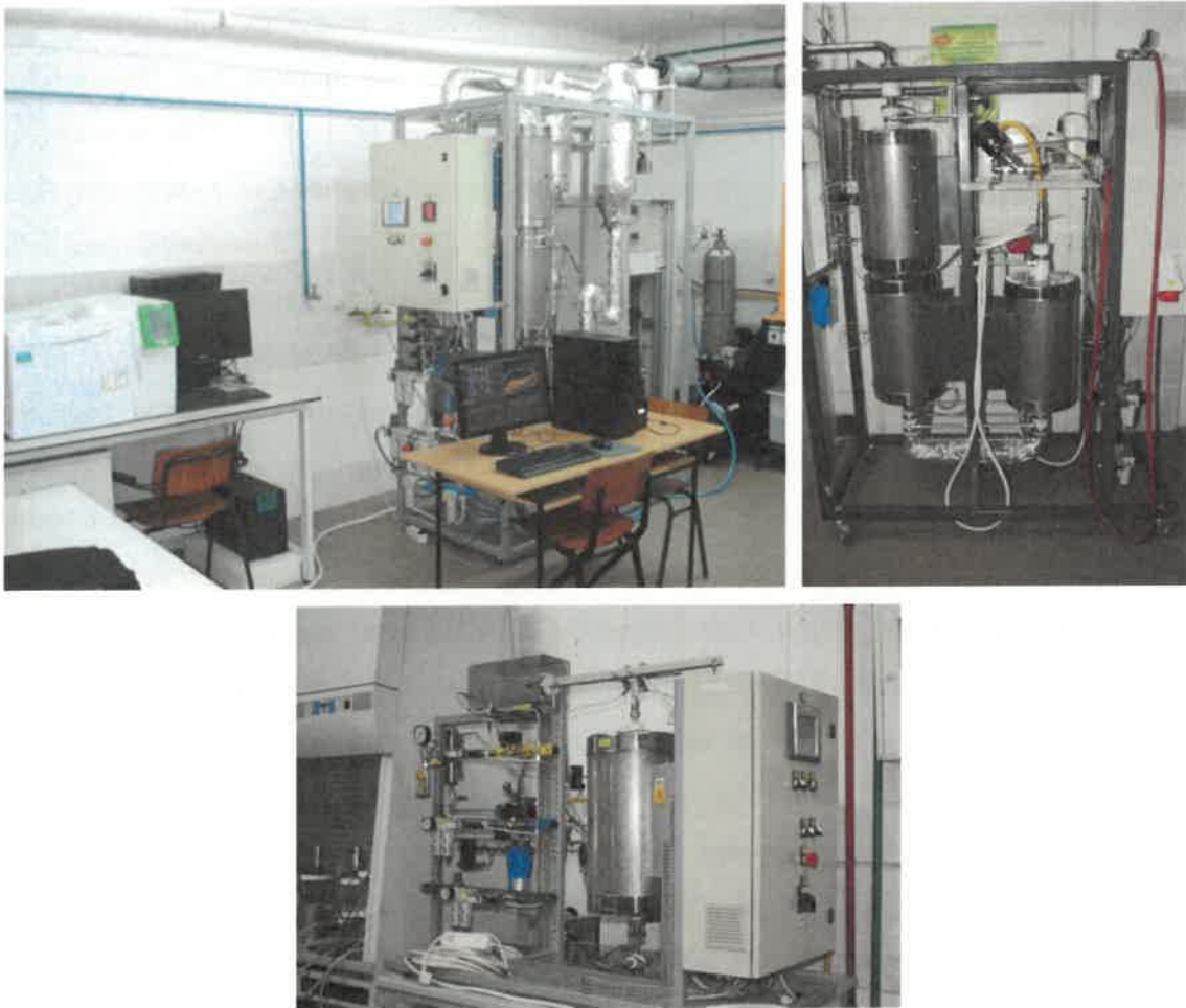
Figure 1. Chemical and calcium looping experimental units developed at Babes-Bolyai University
